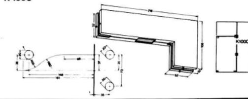
**P-10** Pivot with stainless steel fixing plate
