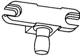
**P-20** Pivot with threaded rod including brass plug
